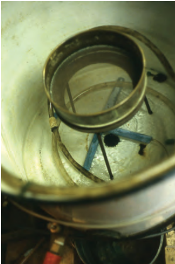
A view inside the flotation tub shows the air stones (blue) and the central screen for capturing the heavy fraction.
