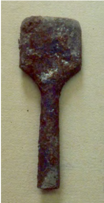
A tapper (left) from the Highland Foundry site was used in preparing sand molds. Identical tappers (right) were in use at the Portland Stove Foundry in 1980.
